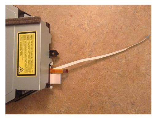
5) Connect the cable from drive daughterboard (FAT/2k/2k1) to MB on the DMC PCB FFC connector, or from PS3 Motherboard to MB connector on DMC for 2k5 and 3k consoles:
