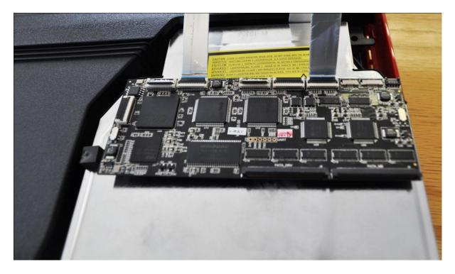
The Cobra ODE should be positioned inside the console as shown (CECH4XXX):
